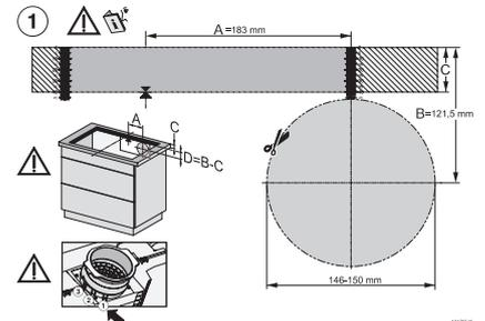
KMDA7272FL, KMDA7473FL – flush installation, drilling template, Installation depth 20 cm, Installation drawing
