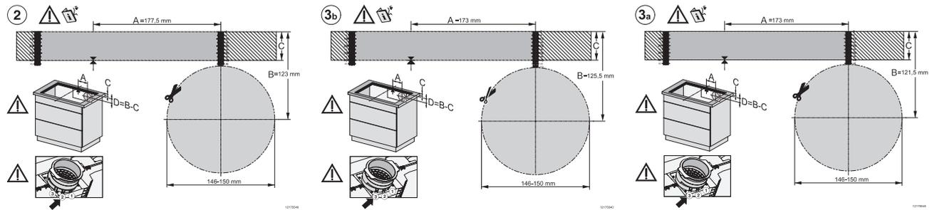
KMDA7272FL/FR, KMDA7473FL/FR – surface installation, drilling template, Installation drawing
